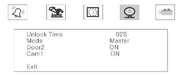
Parameter values of the fourth section of the menu "Monitor operating modes": Unlock time: select the time period during which the signal will be applied to the dry contacts of the call panel, when the lock opening button is pressed (2-10sec).
