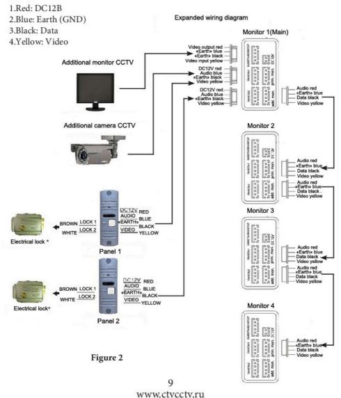
■ The calling panels are connected only to the main monitor. In addition to the two calling panels, an additional camera and a video surveillance monitor (available separately) can be connected to the main monitor. These devices should be switched to the corresponding contacts of the CN5 connector (Fig. 2):\*
