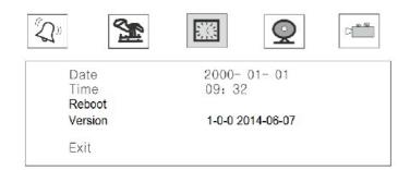
Parameters of the third section of the menu "Date and time settings": Date: sets the current date in the format YYYY-MM-DD.
