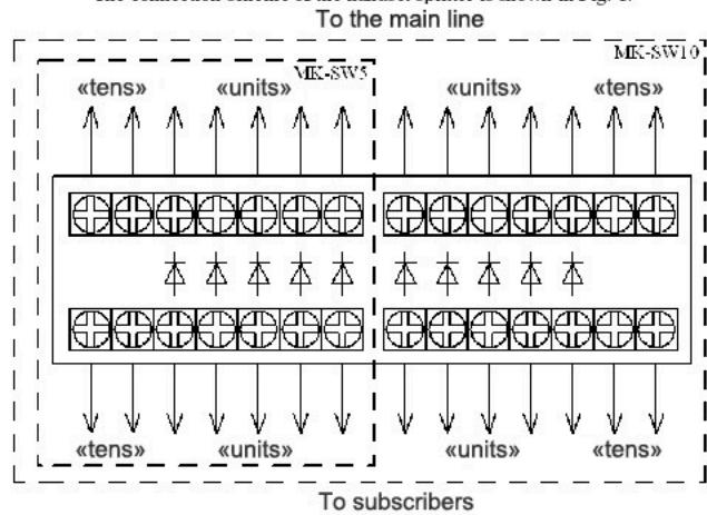
Figure 1. Wiring diagram for METAkom MK-SW10 handset splitter (MK-SW5).
